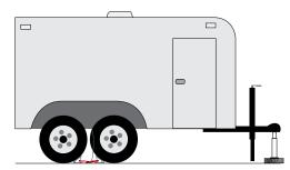
Use a block if needed to raise scale so the trailer can sit parallel to the ground.
